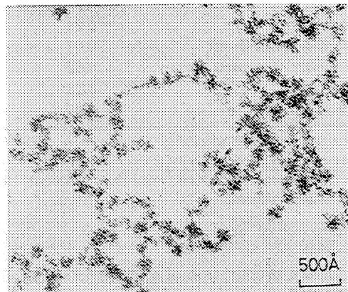
Fig. 1. Electron micrograph of colloidal rhodium dispersion prepared by using \beta -cyclodextrin equimolar to rhodium(III) chloride; \times 100000 .
